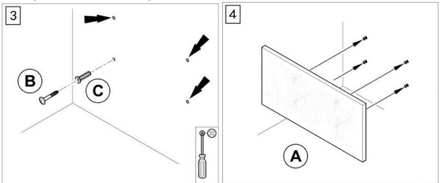
5. Slid the device to make the screws into the correct positions as showing In below drawing.
